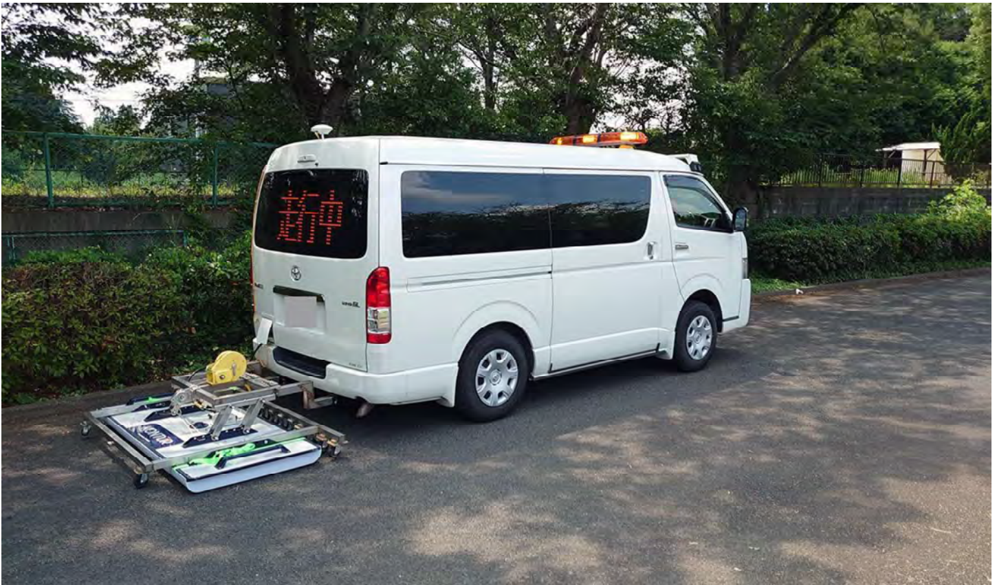
Example of the Ground-DG-1821 System
